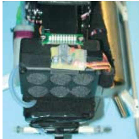
A close up of the Throttle Jockey magnet and sensor orientation
