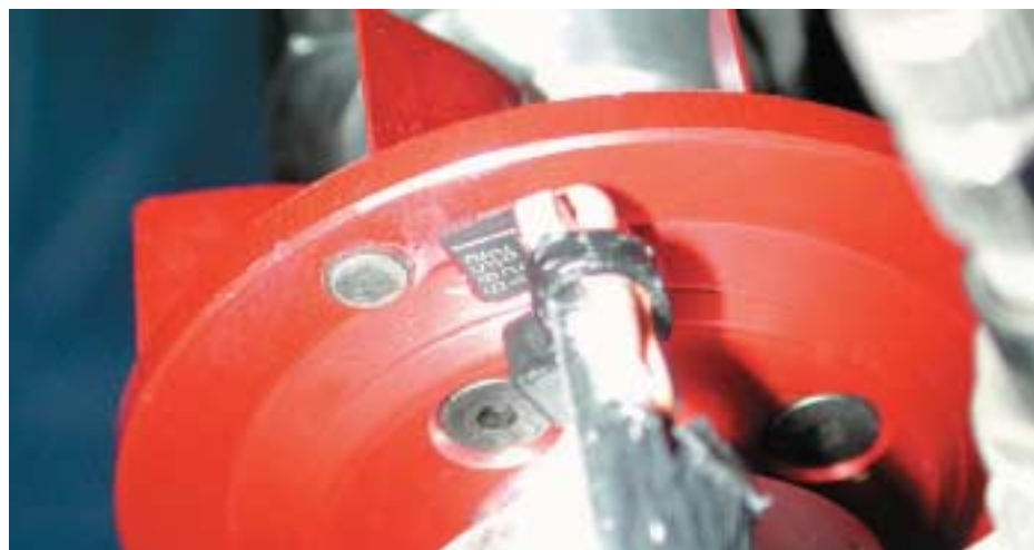
A close up of the Throttle Jockey magnet and sensor orientation
